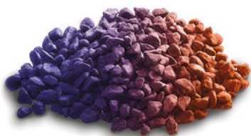
Fig.: EGN 99 granules, with potassium permanganate: new on the left and saturated on the right.
