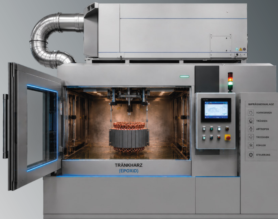
AI-visualised representation of an impregnation system with a ventilation system installed on the roof
