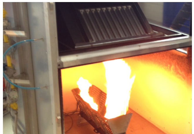
Test rig for assessing the flame-through resistance of separators
