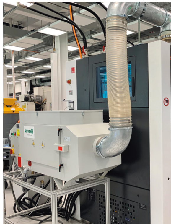
Oil mist separator with coolant return
