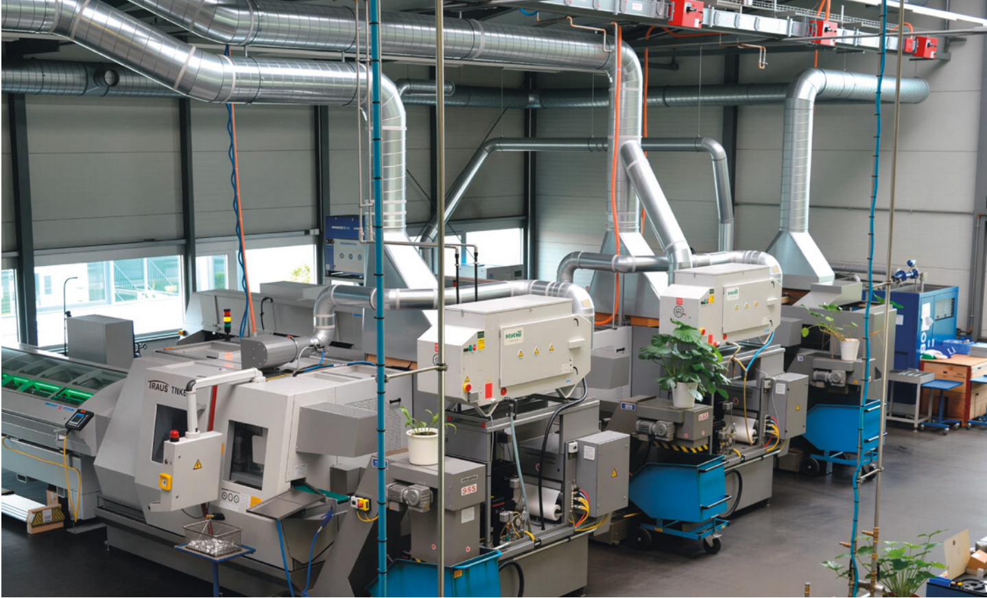
Use of X-CYCLONE® CE-XSC series electrostatic air cleaners in Swiss watch manufacturing
