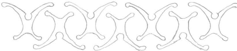
Prototype of the X-CYCLONE® separator with X-shaped profiles modelled on aeroplane wings
