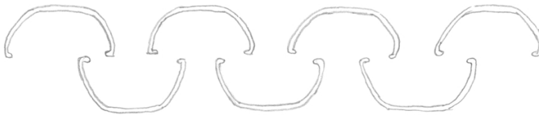
Baffle plate separators with U-shaped profiles
