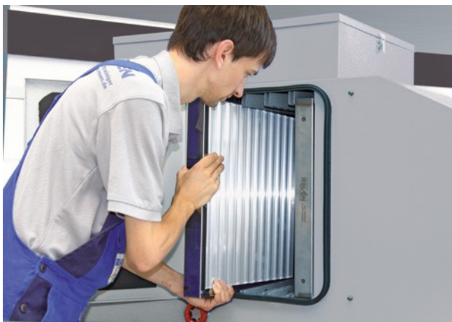
Insertion of a clean X-CYCLONE® separator into an oil mist separator
