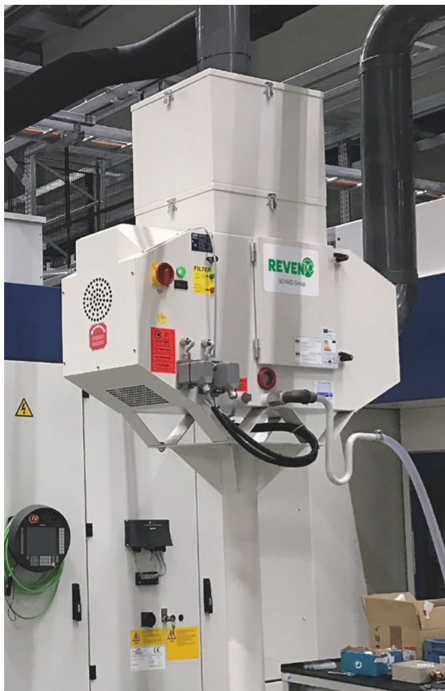
Examples of industrial air cleaners: X-CYCLONE® C (compact air cleaner with additional particulate filter attachment), X-CYCLONE® CE (electrostatic air cleaner), X-CYCLONE® RJ (small compact air cleaner)
