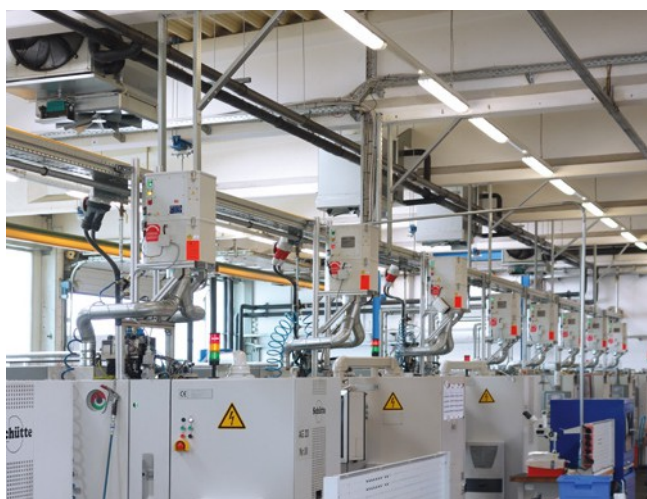
Examples of industrial air cleaners: X-CYCLONE® C (compact air cleaner with additional particulate filter attachment), X-CYCLONE® CE (electrostatic air cleaner), X-CYCLONE® RJ (small compact air cleaner)
