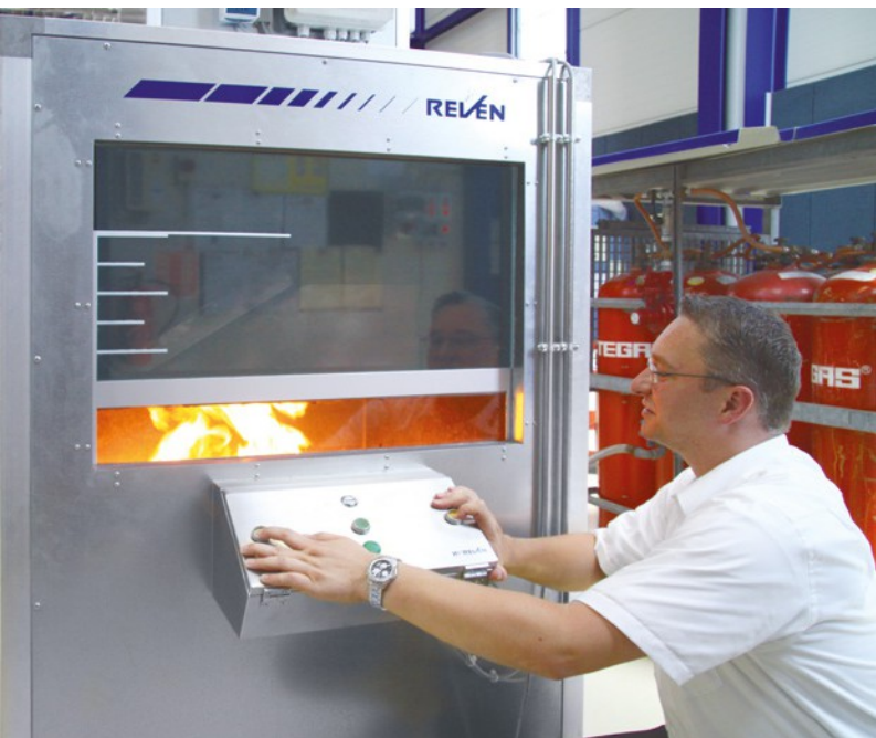
The first testing facility for flame spread resistance in accordance with DIN 18869-5 and DIN EN 16282-6, built by Rentschler REVEN in collaboration with TÜV SÜD Product Service GmbH.
