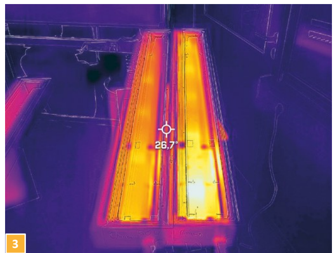
The measuring point on the housing shows a temperature of 26.7 °C
