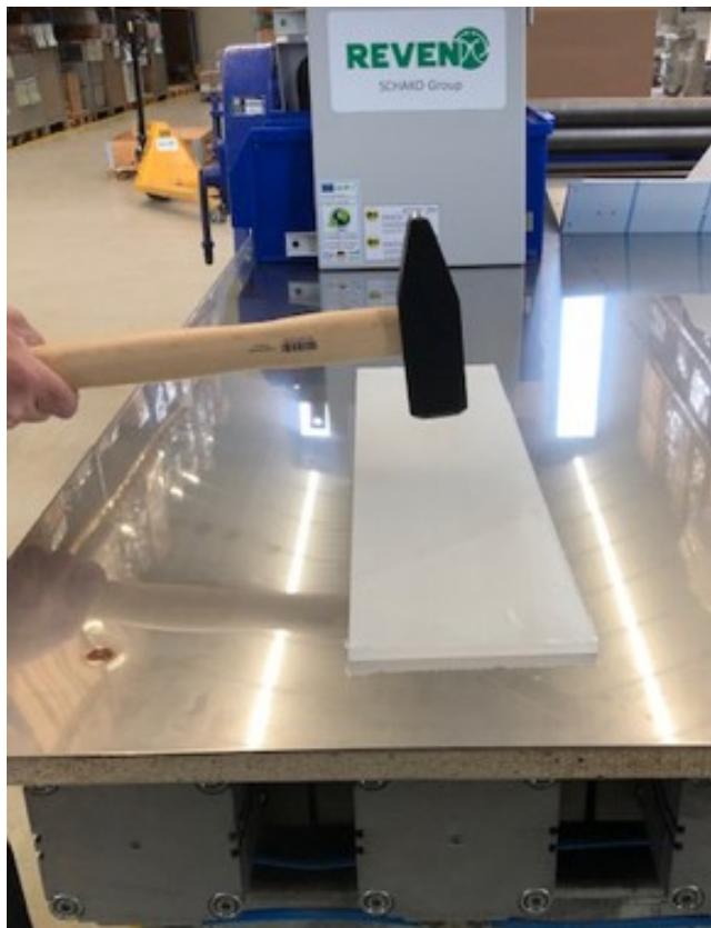
Fig.: Breaking strength test using a 5 kg hammer on the weakest part of the housing, the PLEXIGLAS® cover.
