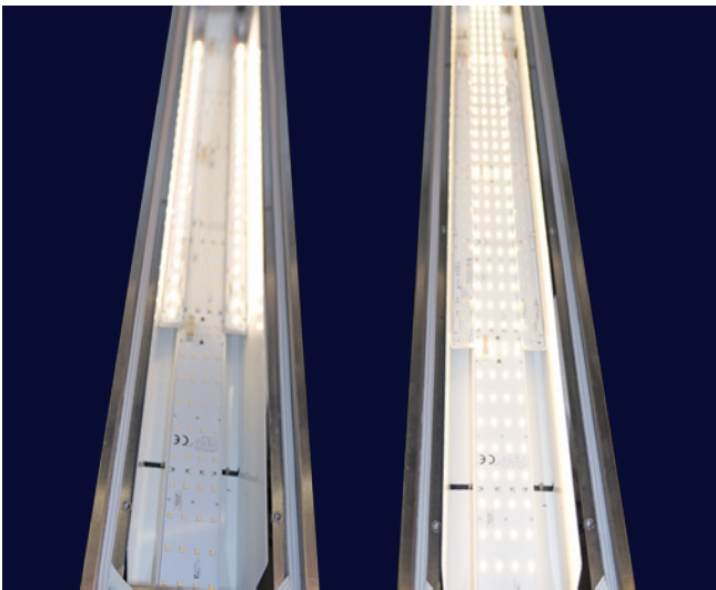
Fig.: On the right, you can see the LED chips on the main circuit boards lighting up. On the left, the LED chips on the additional circuit boards are lighting up.
