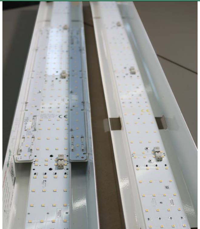
Fig.: The interior mirror has enough space for narrow circuit boards that provide emergency lighting.
