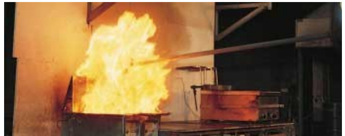
Water is poured into the burning deep fryer using a long pipe. 2cl of water creates a fireball with 1700 times its volume, i.e. 34 litres
