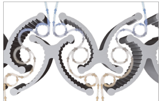
Fig.: Schematic representation of how the X-CYCLONE® Aerosol Separator works
