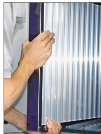
Fig.: When installing the filter, the profiles must be arranged vertically.
