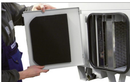
Fig.: The maintenance door can be unhinged to facilitate maintenance operations.
