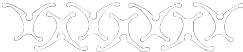
Prototype of the X-CYCLONE® separator with X-profiles in the shape of aircraft wings
