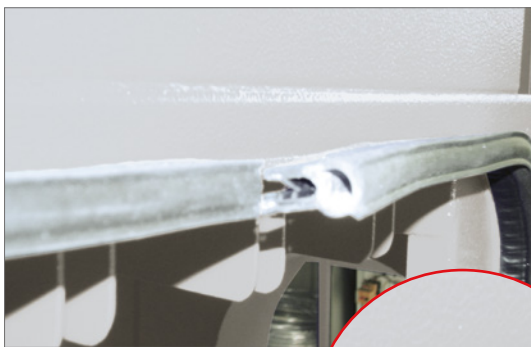
Fig.: Remove the old seal
