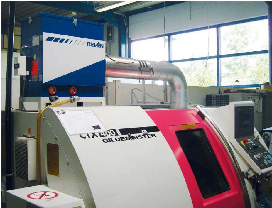
Ill. 8: Separator with Venturi air intake
